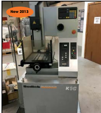
SODICK # K-1C SMALL HOLE EDM "HOLE-POPPER"
