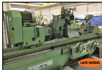
SMTW 20"x 120" CYLINDRICAL GRINDER
