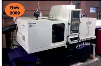
MAIER # MLK-32 "HYBRID" CNC SWISS SCREW MACHINE
