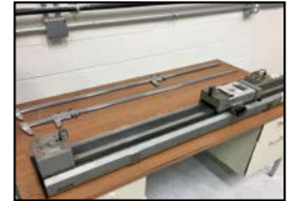
FOWLER-TRIMOS 48" HORIZONTAL SETTING GAGE
