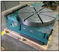
TSUDAKOMA # RNCV-800 CNC "4th-Axis" ROTARY TABLE
