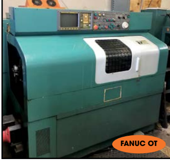
NAKAMURA-TOME # TMC-15 CNC LATHE
