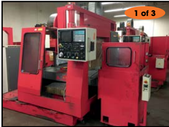
MATSURRA # RA-1 CNC VERTICAL MACHINING CENTER
