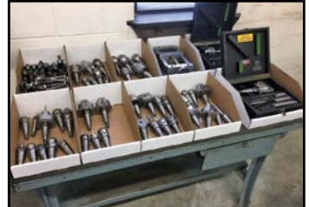
VIEW OF MOORE JIG BORER TOOLING
