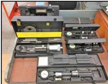
VIEW OF SUNNEN BORE GAGES
