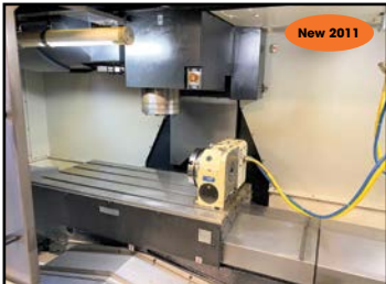
VIEW OF DOOSAN # DNM-500HS CNC VERTICAL MACHINING CENTER INTERIOR w/ KOMA "4th-Axis" Rotary Table
