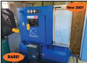
QUINCY # QMB-15 (15 HP) "VARIABLE" SPEED - ROTARY SCREW AIR COMPRESSOR
