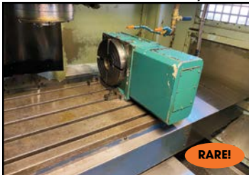
VIEW OF MATSUIURA # MC-800VG-II CNC VERTICAL MACHINING CENTER INTERIOR w/ TSUDAKOMA "4th-Axis" Rotary Table
