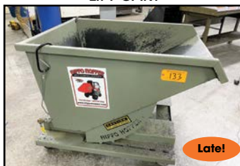
HIPPO-HOPPER SCRAP DUMP HOPPER
