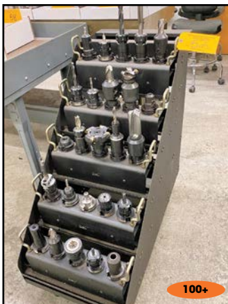
VIEW of #CAT-40 CNC TOOLHOLDERS
