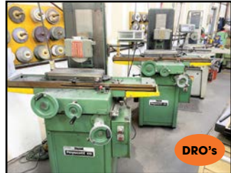
VIEW of SURFACE GRINDERS
