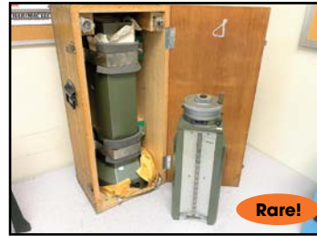
MITUTOYO "HEIGHT-MASTER" GAGE w/ 18" RISER BLOCK
