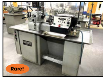
HARDINGE #DV-59 SECONDARY LATHE w/ AIR-CROSS-SLIDE
